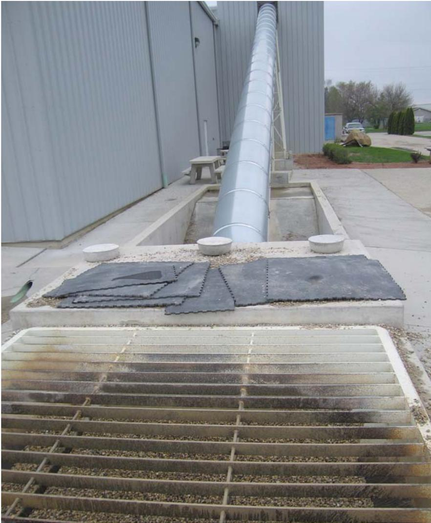
*Below grade aggregate grizzly enables efficient charging of the 2-compartment indoor aggregate silo directly from a truck or frontend loader – no double handling required.*
