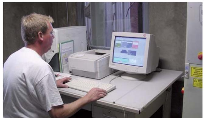
*Dalmaray owner and President Rob Ausen uses the ACT Programmable Control System (PCS) to select recipes, track inventory, and monitor system functions. The PC-based system uses a graphical user interface (GUI) for intuitive control.*
